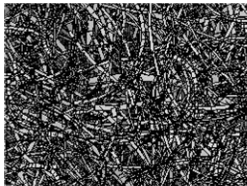
Figure 9. Visualization of simulated paper-like fibre networks with fibres from sawmill chips, left, and from pulpwood, right. The upper images show the surfaces and the thin lower images cross-sections of the networks. Both networks have the same grammage, g/m^2 , and the same sheet density, kg/m^3 .
