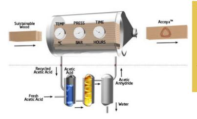
Acetylation is a method of chemical modification where acetyl groups are bound to reactive sites in the wood. This makes the wood more resistant to decay and movement due to moisture. The method has for been considered wood processing for several decades but it is only recently that sufficient technological advances have allowed feasible commercialisation.
