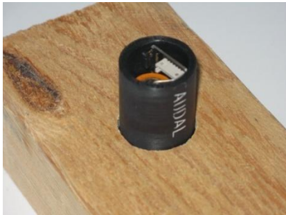
Fig 5. & 6. Cadix sensor's easy and wireless installation.
