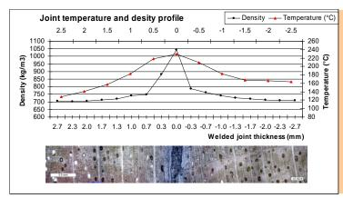
Linear welding results in an extremely localised effect, where the molten region is limited to the immediate region of the weld interface. The molten region causes cell wall collapse and densification within this local region, resulting in a dense region around the weld. Correct processing will result in a strong wood-wood bond, without the use of adhesives. Work is continuing to understand the welding process.
