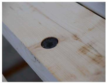
Illustration. Lignin glue testing. Knot reparation. PHOTOS: RGBSTOCK, CHIMAR
