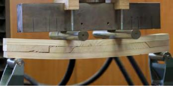
Lignin based glue testing. Eco-beam testing. PHOTOS: AIDIMA, CBD
