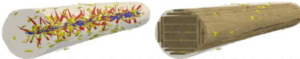
Figure 2. Left: Log with automatically detected features; sound knots (yellow), dead knots (red), splits (blue) and resin pockets (yellow). Right: Virtual break-down of log into boards.
