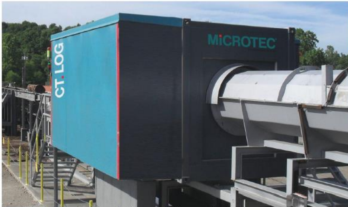
Figure 1. The first installation of a high-speed CT scanner for logs.
