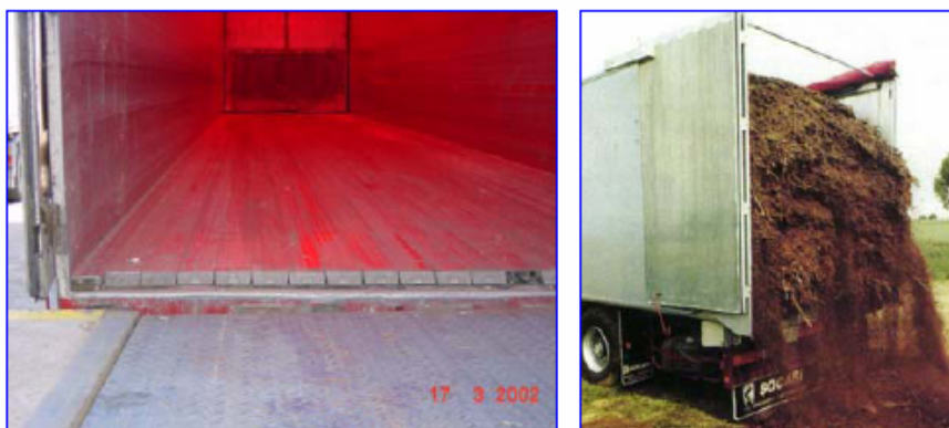
Figure 11 – Scrapper floor for chips unloading
