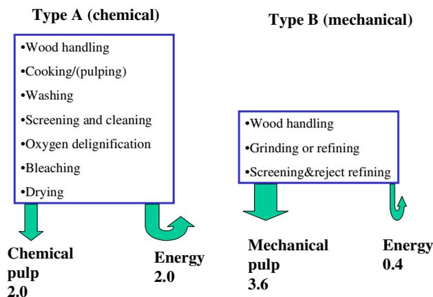
3. In the next step wood is converted into pulp. The two main types of pulping, mechanical and chemical, differ substantially in output of the pulp and energy consumption. Again, the other indicators not discussed here, may differ as well.
